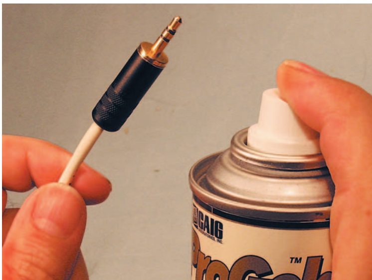
Figure 3.3.46 Spraying with ProGold.
