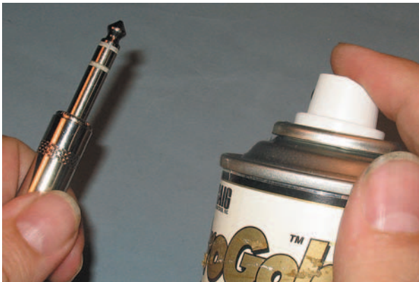
Figure 3.1.51 Spraying with ProGold.
