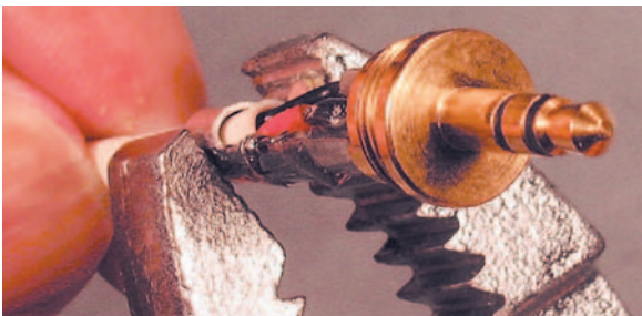
Figure 3.3.39 Clamping yoke onto wire – 3.
