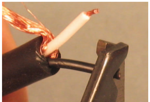
Figure 3.2.23 Stripping low conductor.
