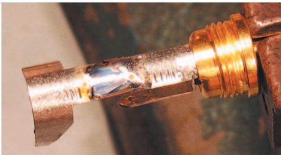
Figure 3.3.24 Correct tinning of strain relief.
