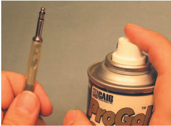
Figure 3.7.68 Spraying with ProGold.
