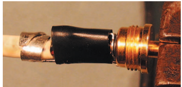
Figure 3.3.44 Tape wrap completed.
