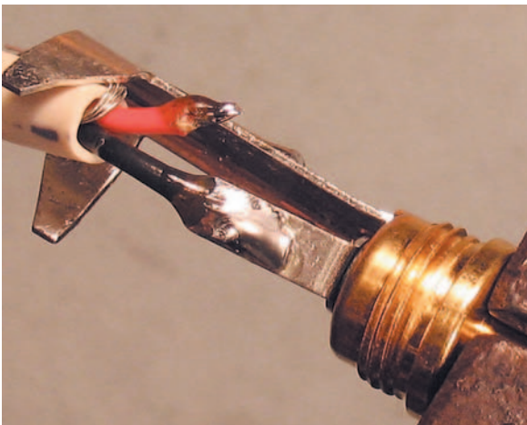
Figure 3.3.27 Finished low conductor joint.
