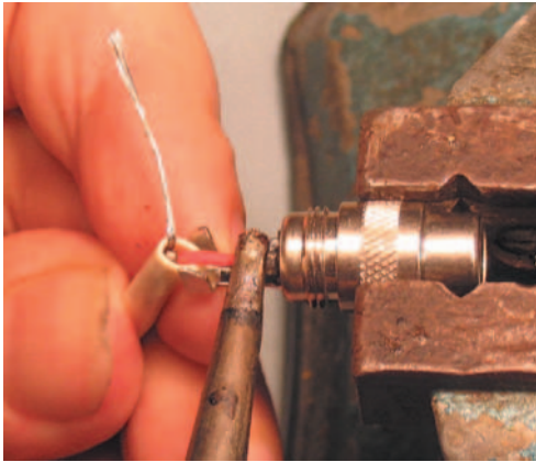
Figure 3.5.25 Attaching high conductor – 2.
