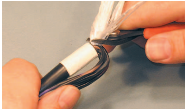
Figure 1.73 Cutting away insulation/wrapping.
