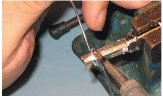
Figure 3.1.21 Tinning strain relief.
