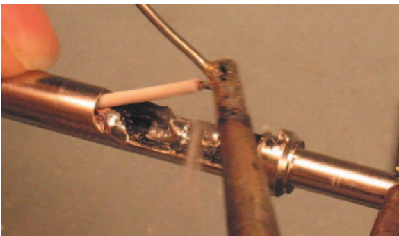
Figure 3.7.55 Tinning high conductor.
