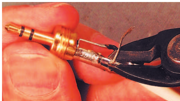
Figure 3.3.36 Removing excess drain strands.
