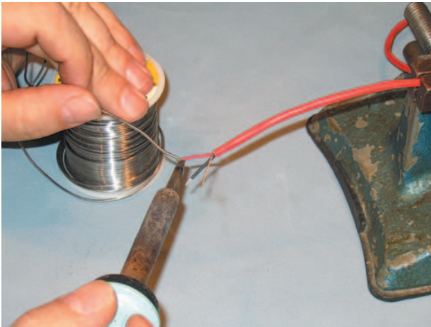
Figure 1.80 Tinning inner conductors.
