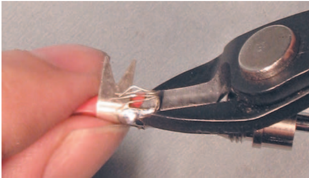
Figure 3.4.30 Cutting excess drain.
