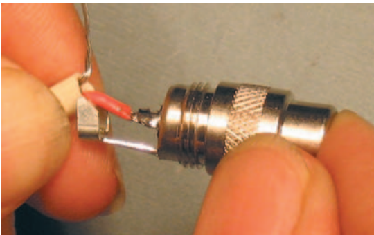
Figure 3.5.26 Completed high conductor.
