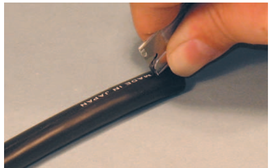
Figure 1.67 Continuing cut with slitter – 2.
