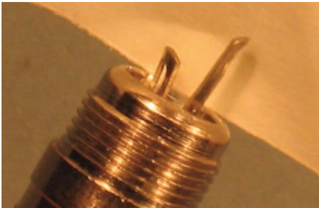
Figure 3.2.31 Flaring solder tabs – 2.
