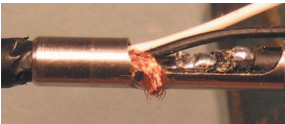
Figure 3.7.37 Excess shield cut.
