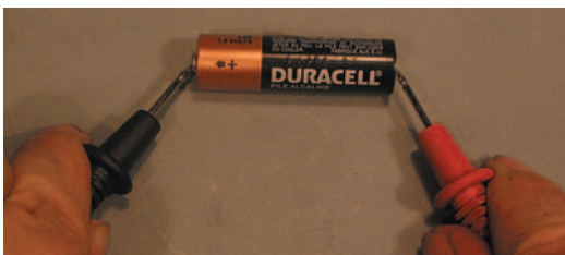
Figure 2.2.23 Test AA battery.
