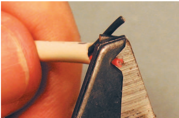
Figure 3.3.11 Stripping conductor ends.
