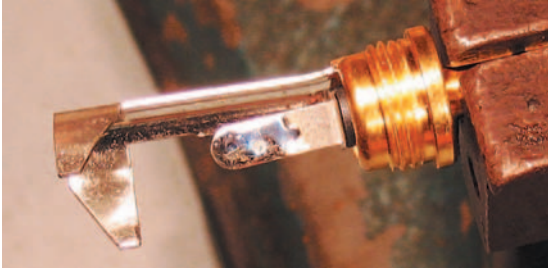
Figure 3.3.20 Correct low tab tinning.
