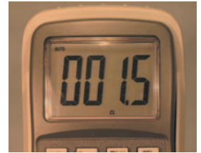
Figure 2.2.17 Twenty-foot cable resistance.
