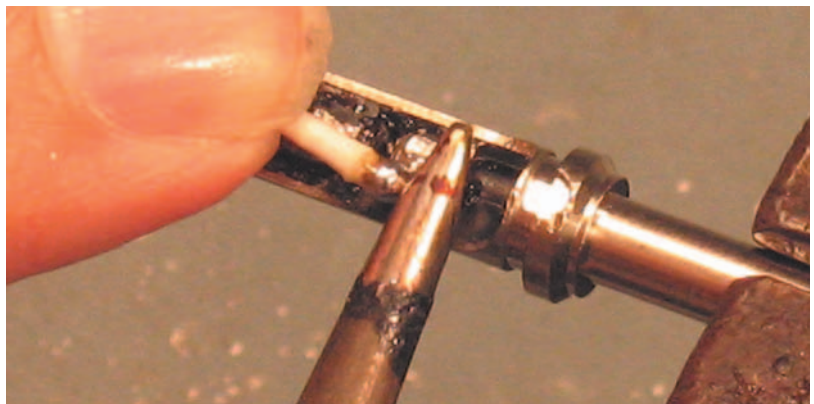
Figure 3.7.58 Solder high conductor.
