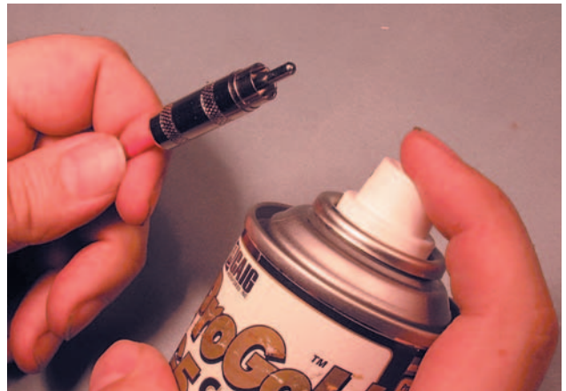
Figure 3.4.34 Spray the RCA with enhancer.
