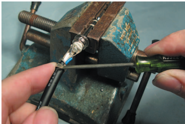
Figure 1.86 Mount plug and open strain relief.
