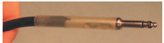
Figure 3.7.65 Second heat-shrink layer.
