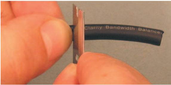
Figure 3.7.6 Cut outer jacket with razor blade.
