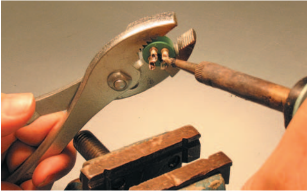
Figure 1.84 Heating solder cups.
