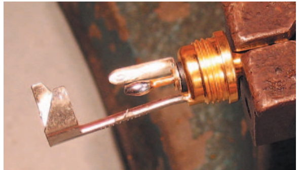
Figure 3.3.22 Correct high tab tinning.
