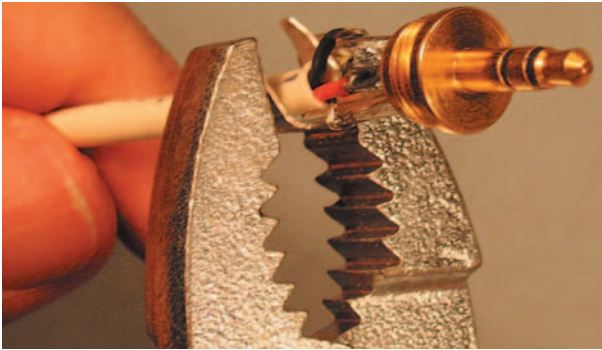
Figure 3.3.37 Clamping yoke onto wire – 1.
