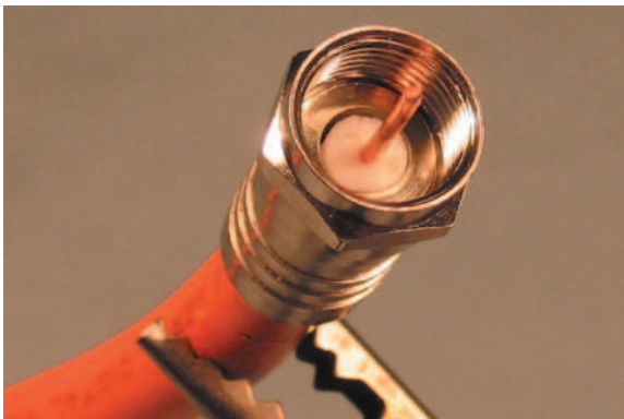
Figure 3.9.5 Wire in place.
