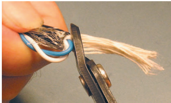
Figure 3.1.14 Cutting away insulation.
