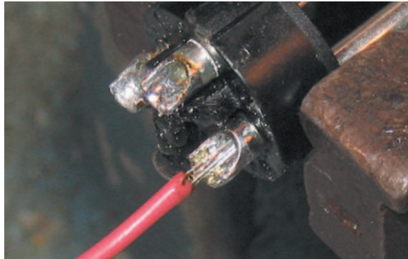
Figure 2.1.2 Too little solder.
