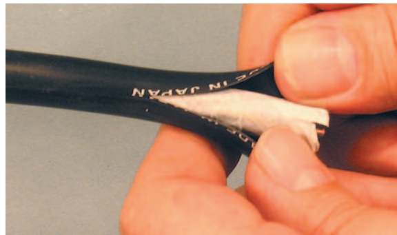
Figure 1.69 Peeling back outer jacket.
