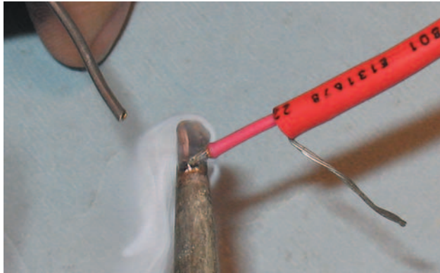
Figure 3.4.19 Tinning high conductor.
