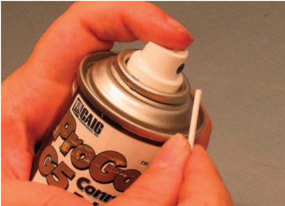
Figure 3.6.42 Spray shaft of Q-tip.
