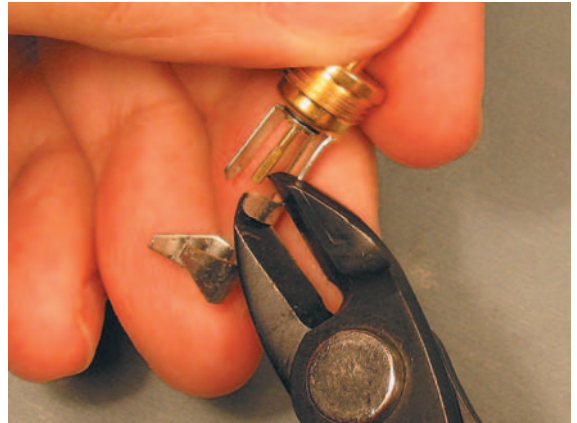
Figure 3.3.17 Cutting off solder tab.
