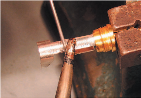
Figure 3.3.23 Tinning strain relief arm.
