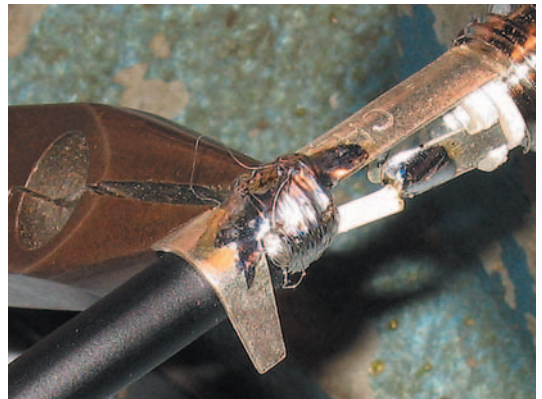
Figure 3.1.43 Correctly soldered shield.
