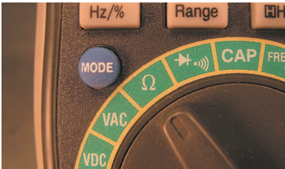
Figure 2.2.6 Set to ohms function.
