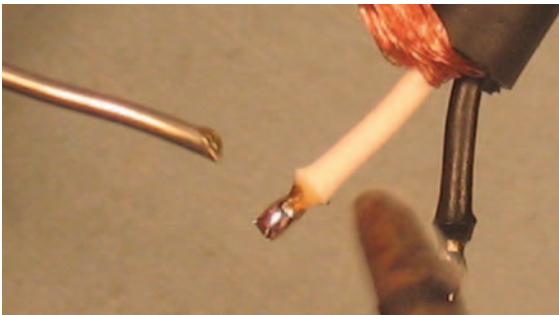
Figure 3.2.27 Beading high conductor – 2.
