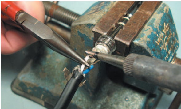
Figure 1.87 Removing soldered conductors.
