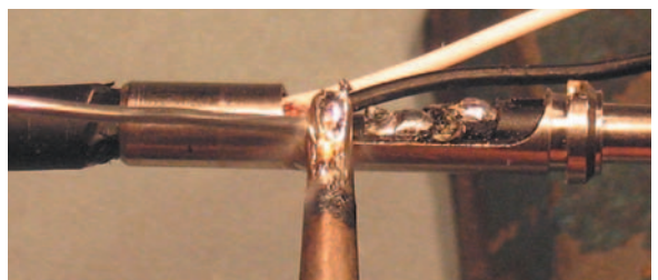
Figure 3.7.38 Solder shield strands.
