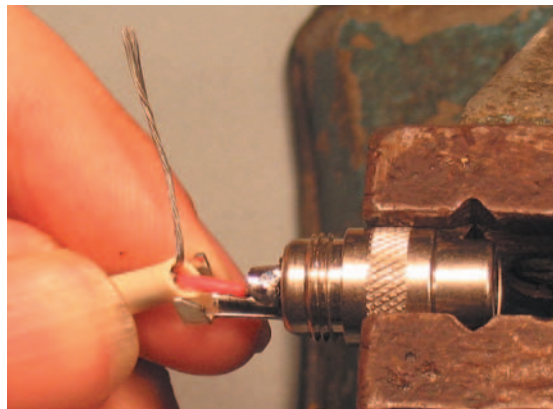
Figure 3.5.24 Attaching high conductor – 1.
