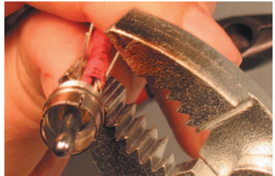
Figure 3.4.33 Crimping strain relief.
