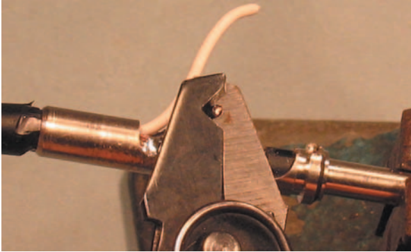
Figure 3.7.44 Stripping low conductor – 1.
