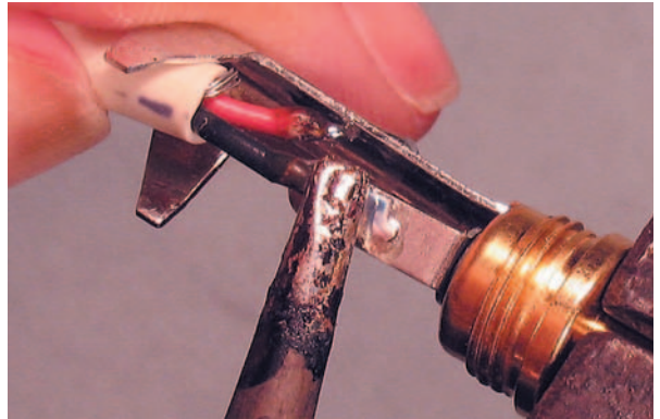
Figure 3.3.26 Soldering low conductor.
