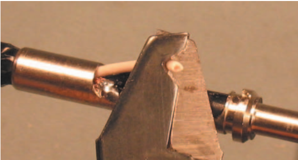
Figure 3.7.53 Stripping high conductor.
