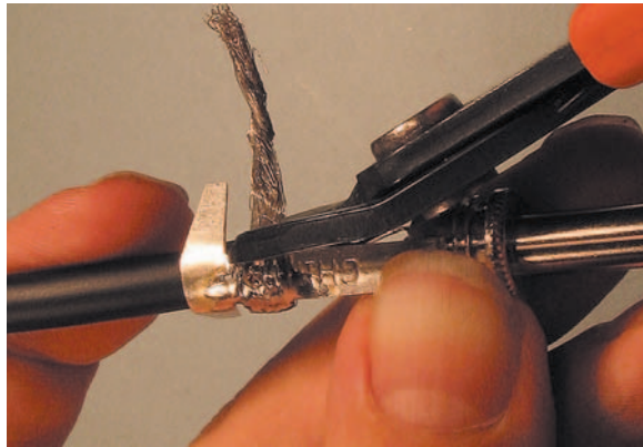
Figure 3.1.44 Cutting excess shield strands.
