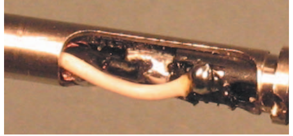
Figure 3.7.60 Soldered high conductor – 2.
