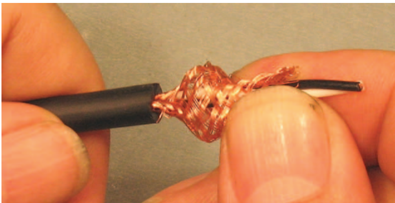
Figure 3.2.11 Push shield conductor strands back.
