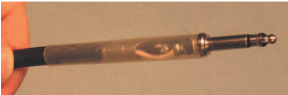
Figure 3.7.62 First layer of shrink.
