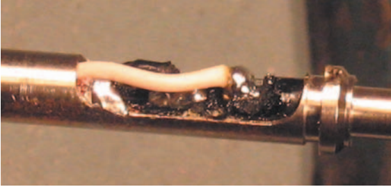
Figure 3.7.59 Soldered high conductor – 1.
